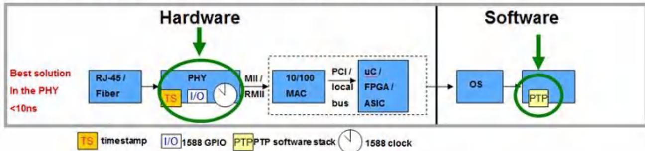
Figure 3. Hardware Time-stamp Block Diagram
