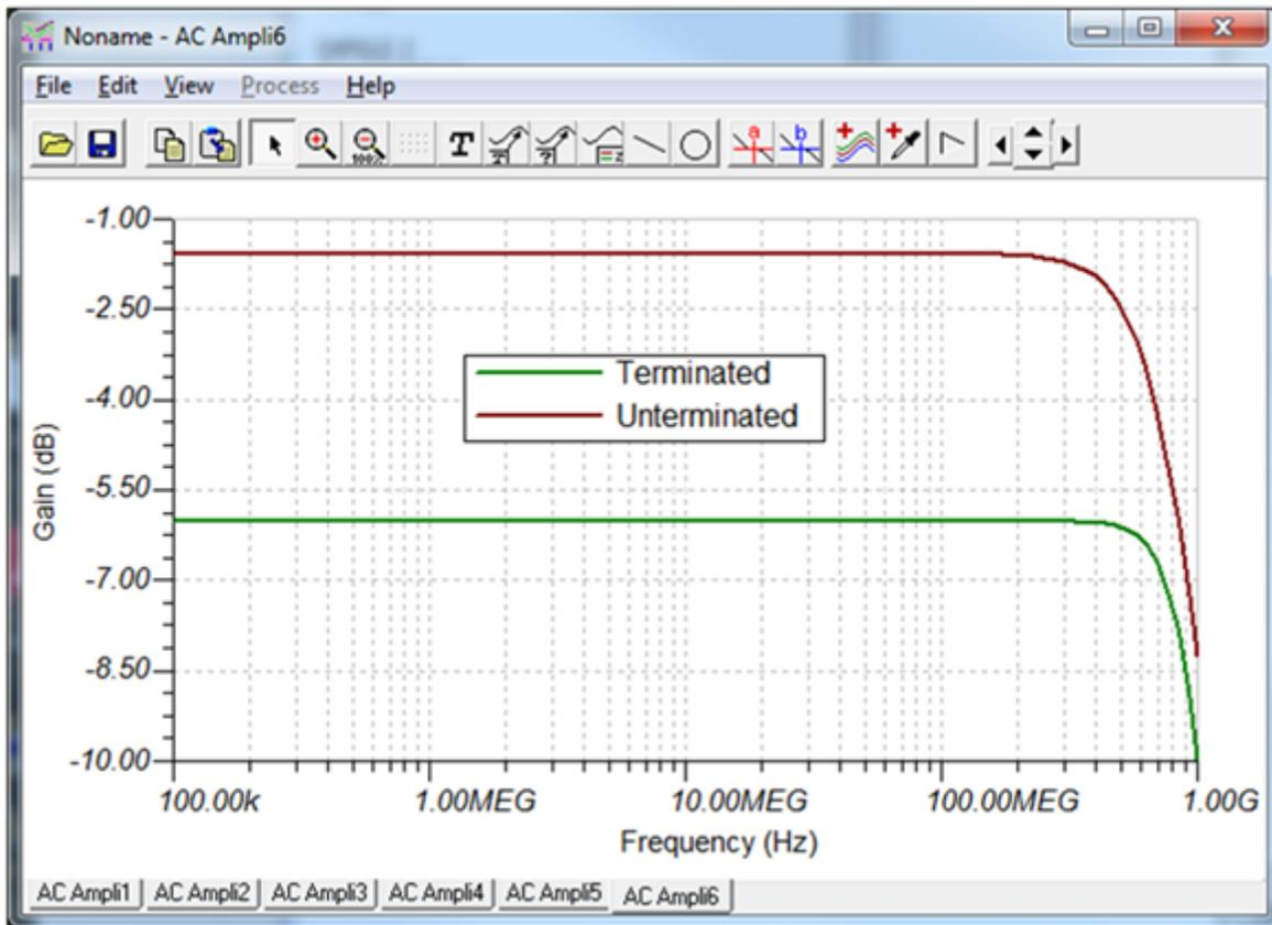
Figure 6. Results with Different Driving Impedances
