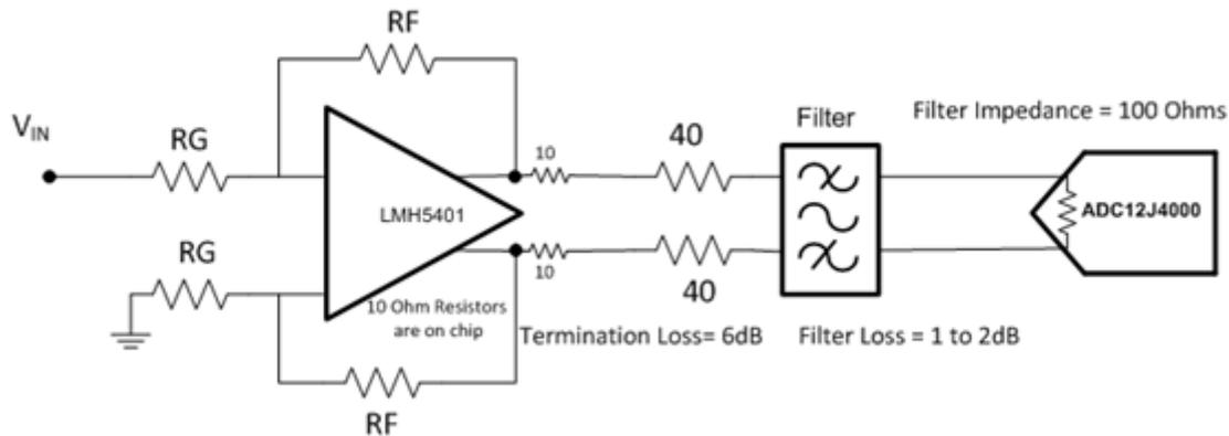
Figure 1. Typical Signal Chain
