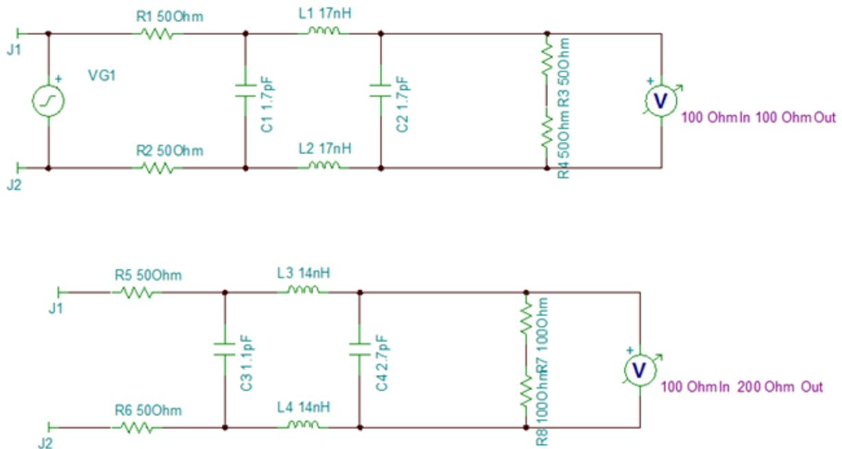
Figure 3. Filters with Different Impedance Ratios
