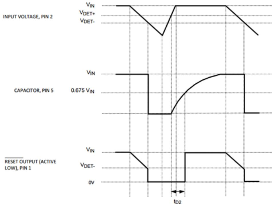
**Figure 2. Timing Diagram for the LM8365**
