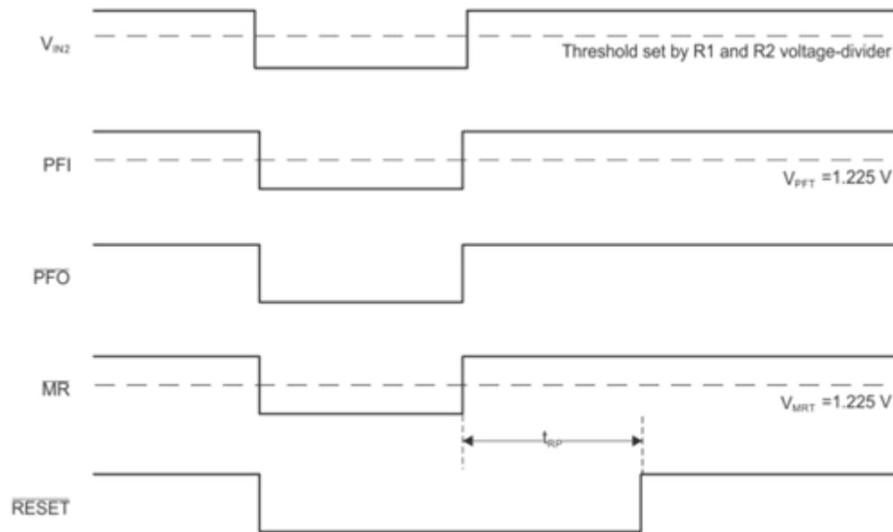
**Figure 4. Example Timing Diagram for Power-fail and Manual Resets of the LM3710**
