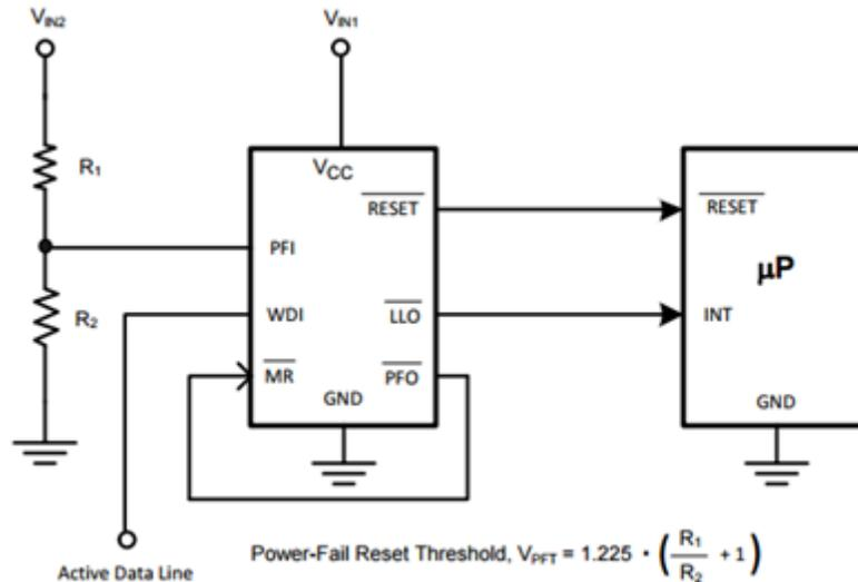
**Figure 3. LM3710 Application Circuit**
