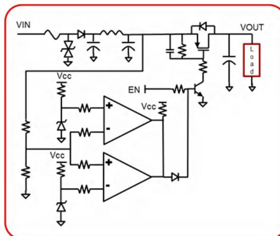
Figure 1. Discrete Protection Scheme
