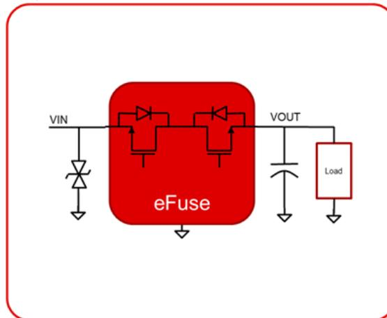
**Figure 3. Integrated Protection Scheme**
