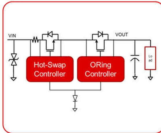
**Figure 2. Controller + MOSFET Protection Scheme**
