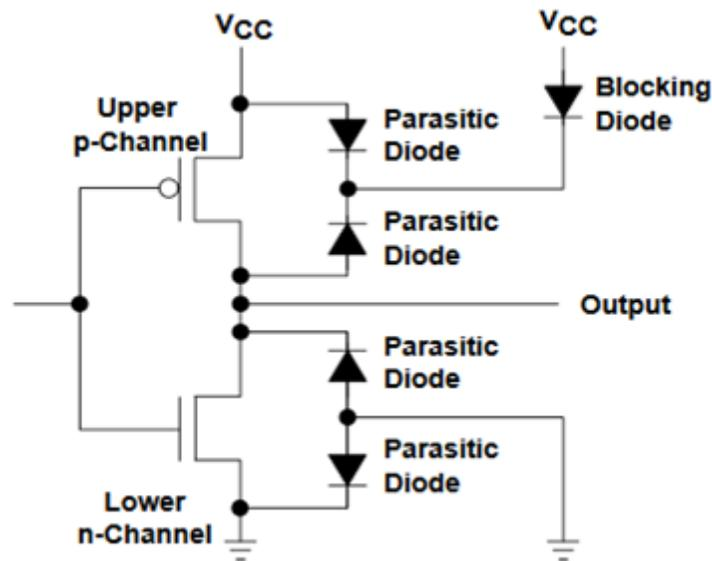
**Figure 3. Typical Powered-off Protection Circuit**
