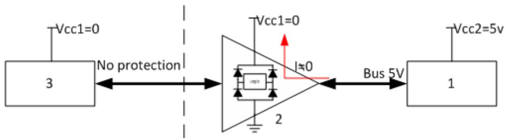
**Figure 1. Device without Powered-off Protection**
