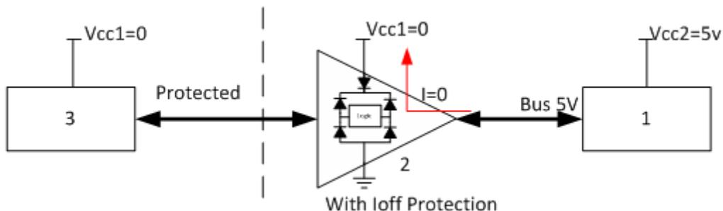
**Figure 2. Device with Powered-off Protection**
