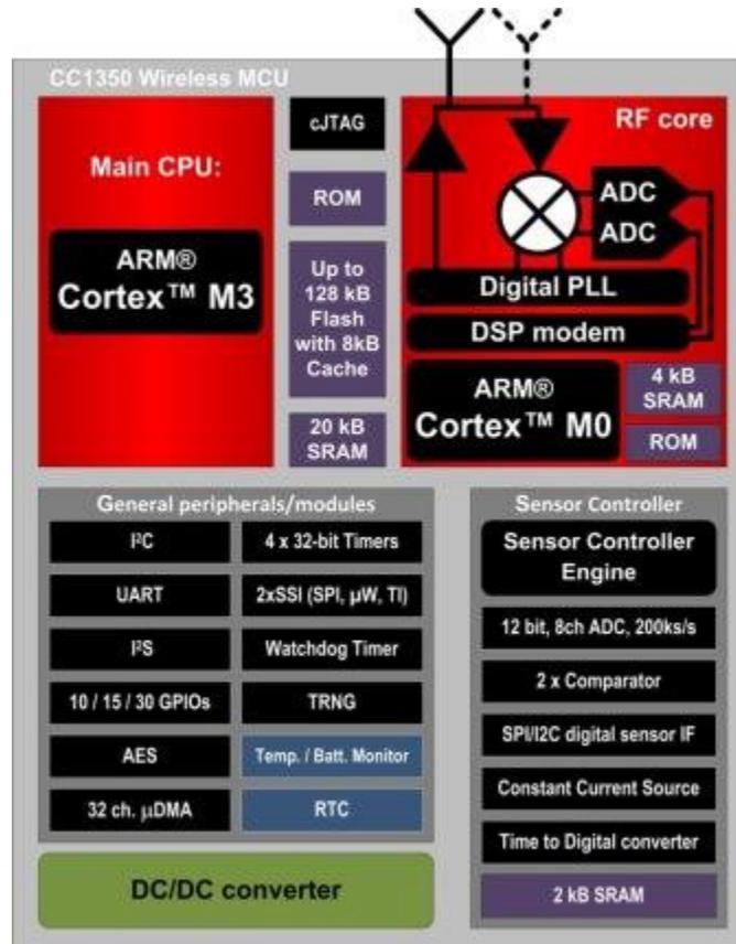
Figure 1. Block Diagram of the SimpleLink Dual-band CC1350 Wireless MCU
