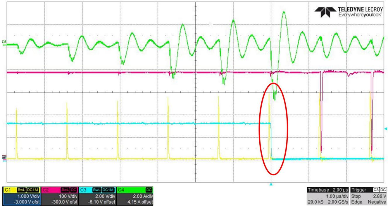
**Figure 2. An TI LMG3410 Shoot-through Test on an LLC Series Resonant Half-bridge Converter:**
