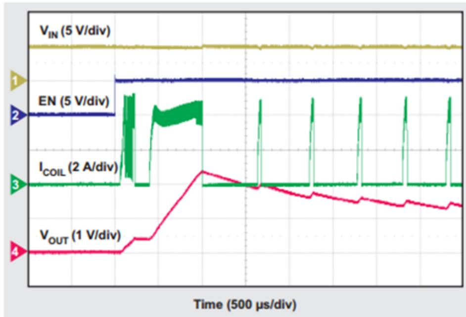
**Figure 1. Because of This FPGA's High Startup Load and Very-High Decoupling Capacitance, the DC/DC Converter Cannot Bring Its Output Voltage into Regulation**
