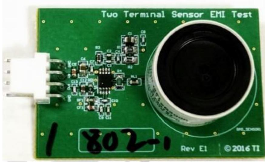
**Figure 2. Test Board with Sensor**
