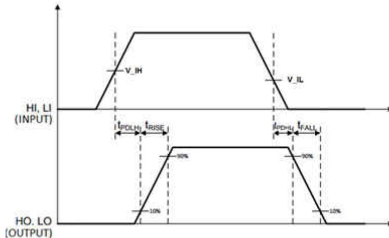
**Figure 1. Typical Rise and Fall Time Diagram**
