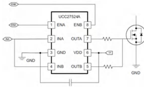
**Figure 2. The UCC27524A with Paralleled Outputs to Double Drive-current Capability**
