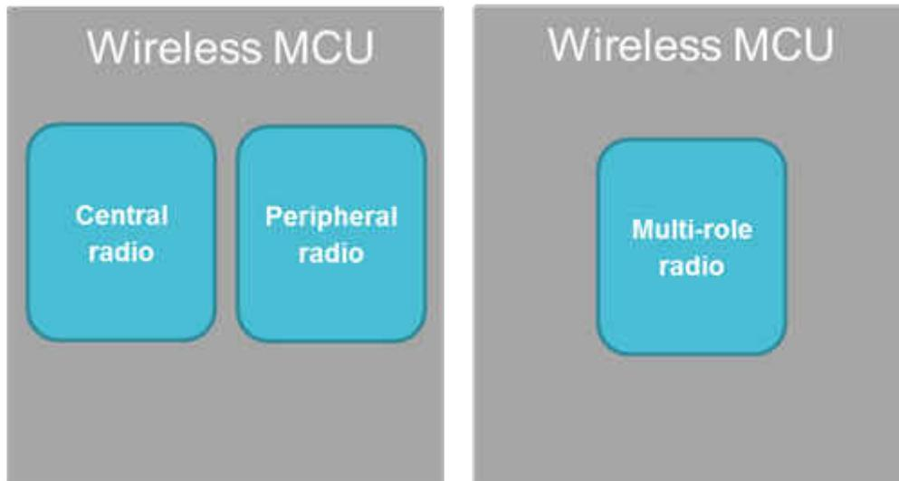
**Figure 2. Bluetooth® low energy Wireless MCU Without and With Multi-role**
