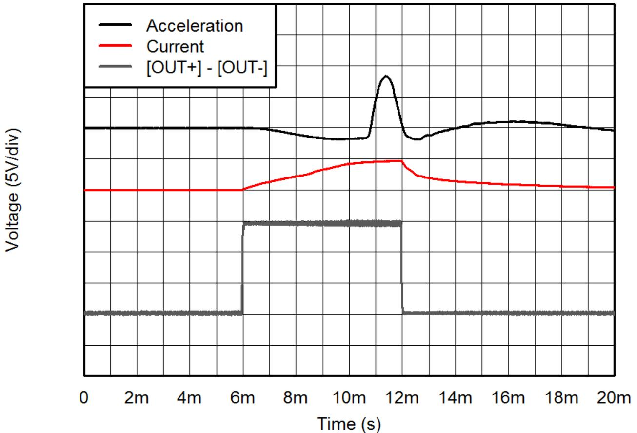
Figure 1. Solenoid Acceleration Graph: Acceleration = 5.85G/div; Current = 2A/div; Voltage = 5V/div
