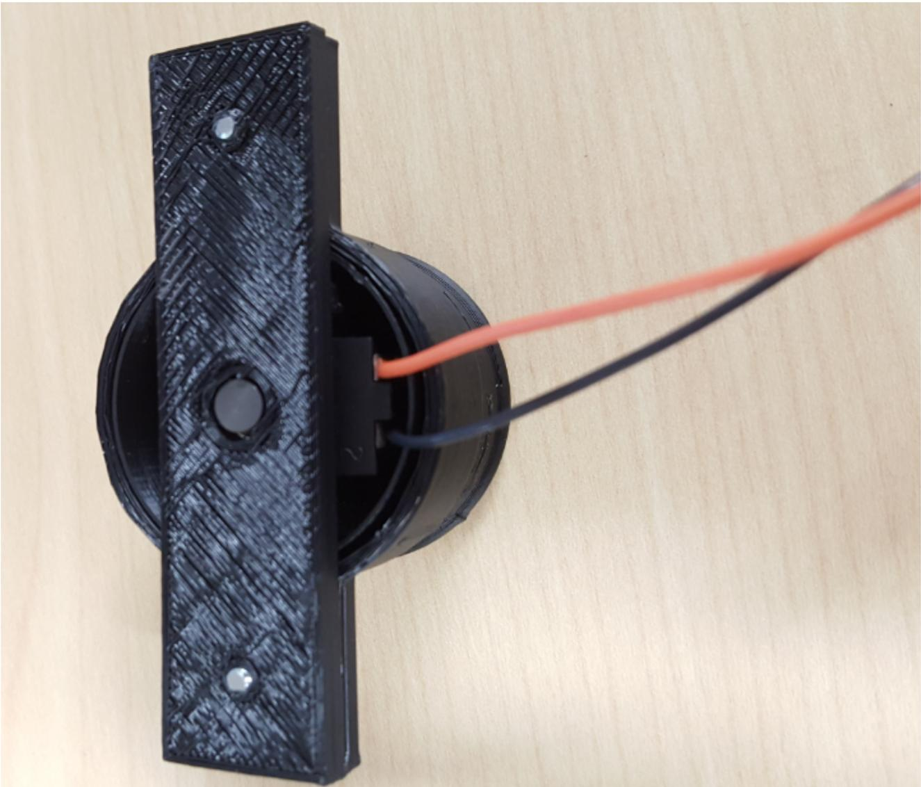
**Figure 2. 3D Printed Solenoid Knob**
