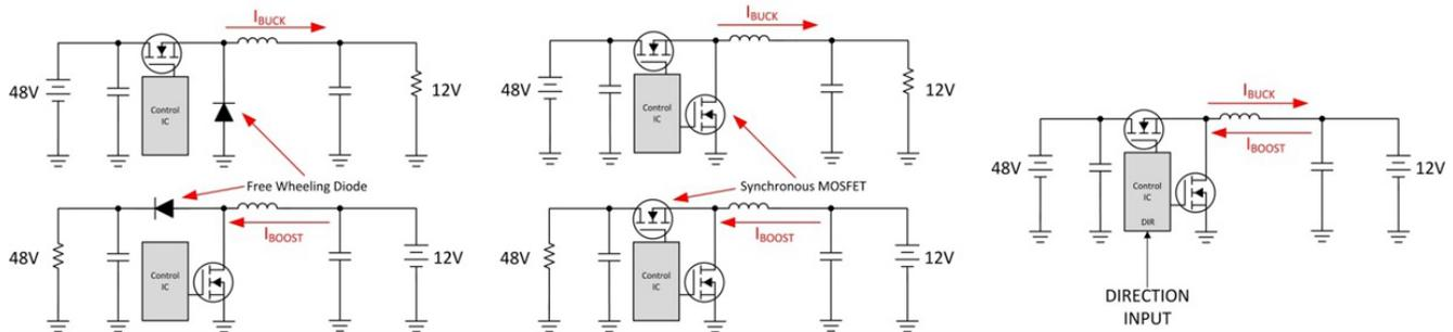
**Figure 2. Evolution of a Single Controller Bidirectional Converter**
