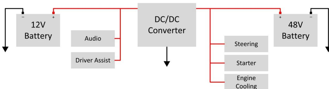
**Figure 1. Block Diagram of a Dual-battery Automotive System**
