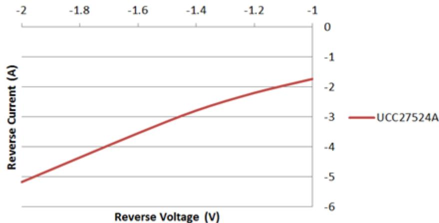
Figure 1. Negative Reverse Voltage Handling
