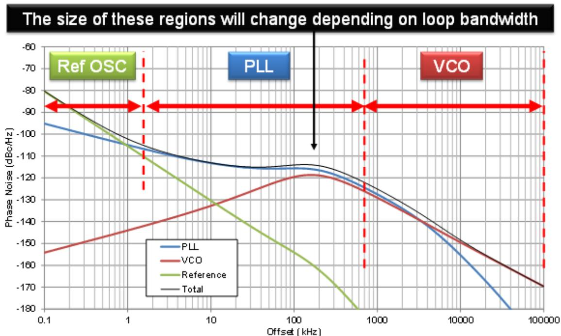
**Figure 3. Typical Phase Noise of a PLL with a Wide Loop Bandwidth**
