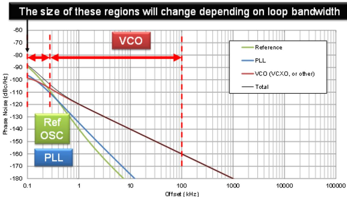
**Figure 4. Typical Phase Noise of a PLL with a Narrow-loop Bandwidth**
