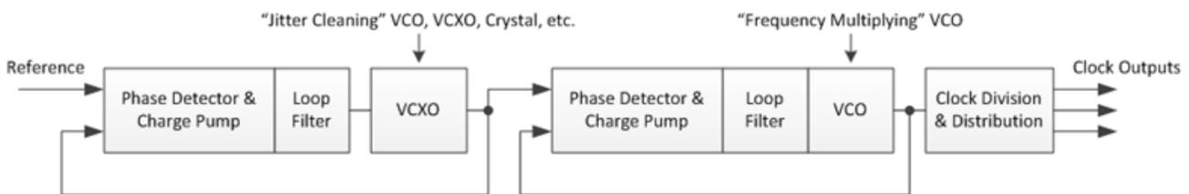
Figure 2. Dual-loop Jitter Cleaner
