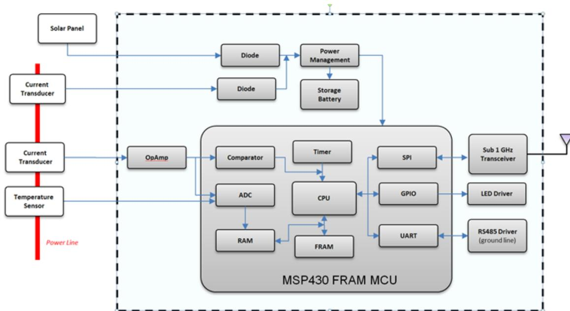
**Figure 2. Functional Block Diagram of a Smart Fault Indicator Based on the MSP430 FRAM MCU**
