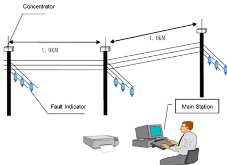
**Figure 1. A Smart Fault-indicator System**
