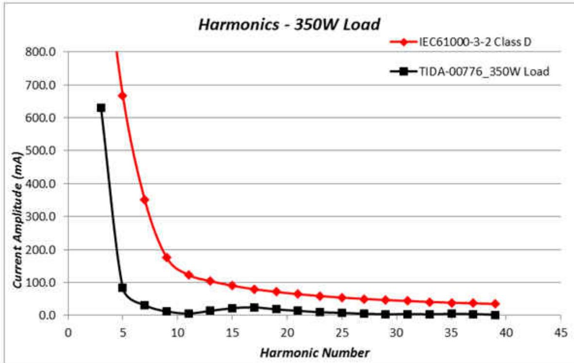
Figure 8. Current Harmonic for 350W Output Power
