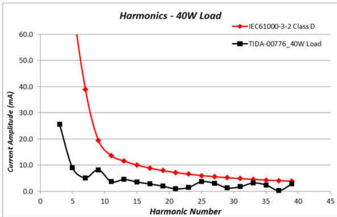
**Figure 6. Current Harmonic for 40W Output Power**
