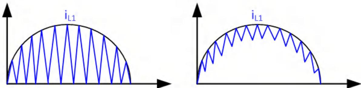
Figure 5. TM PFC (a); Continuous Conduction Mode PFC (b)
