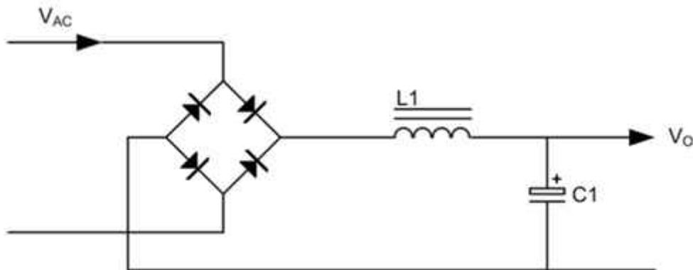
**Figure 2. Typical Passive PFC with Inductor Compensation**
