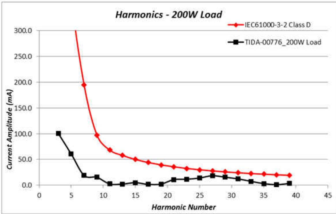
Figure 7. Current Harmonic for 200W Output Power
