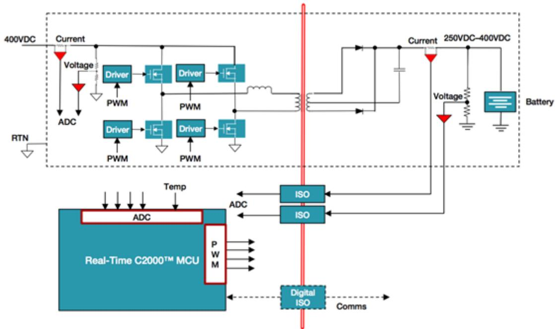
Figure 2. C2000 MCU Controlling a Full-Bridge LLC DC/DC
