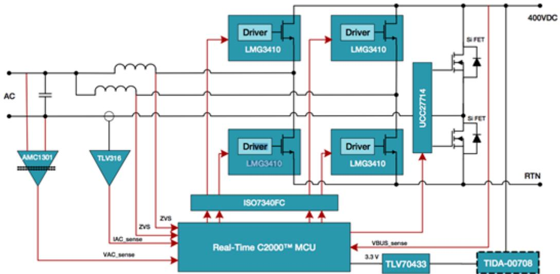
Figure 1. C2000™ MCU Controlling a Two-Phase Interleaved Totem-Pole PFC
