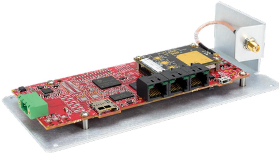
**Figure 1. FreeWave's Newest 900 MHz, FHSS Data Radio, the Z9-P. Offers Programmability for True Edge Intelligence. Also, Available in Ruggedized Enclosure.**
