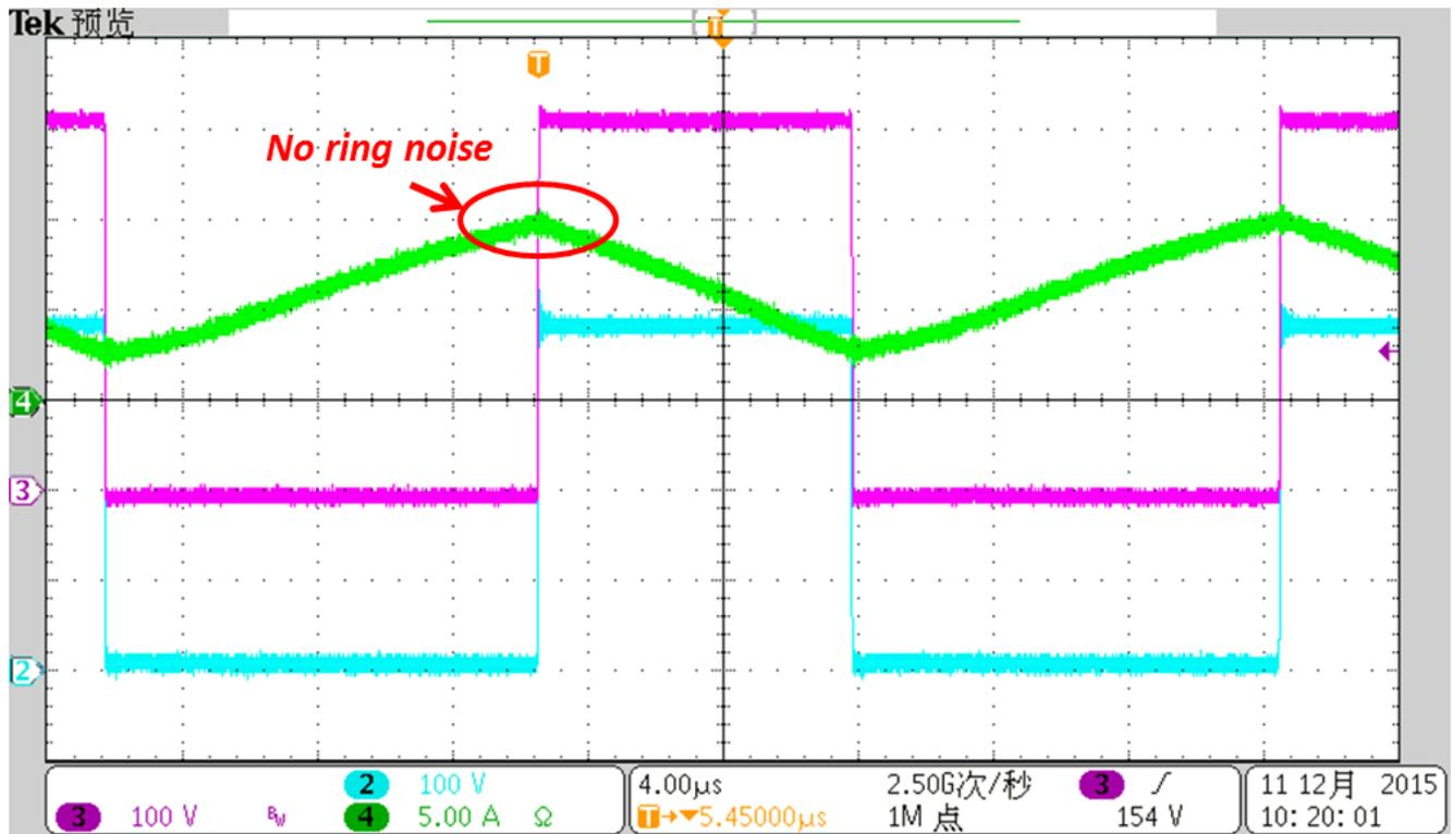
**Figure 3. Switching-Frequency PFC Choke Current Under a 230-V<sub>AC</sub> Input**
