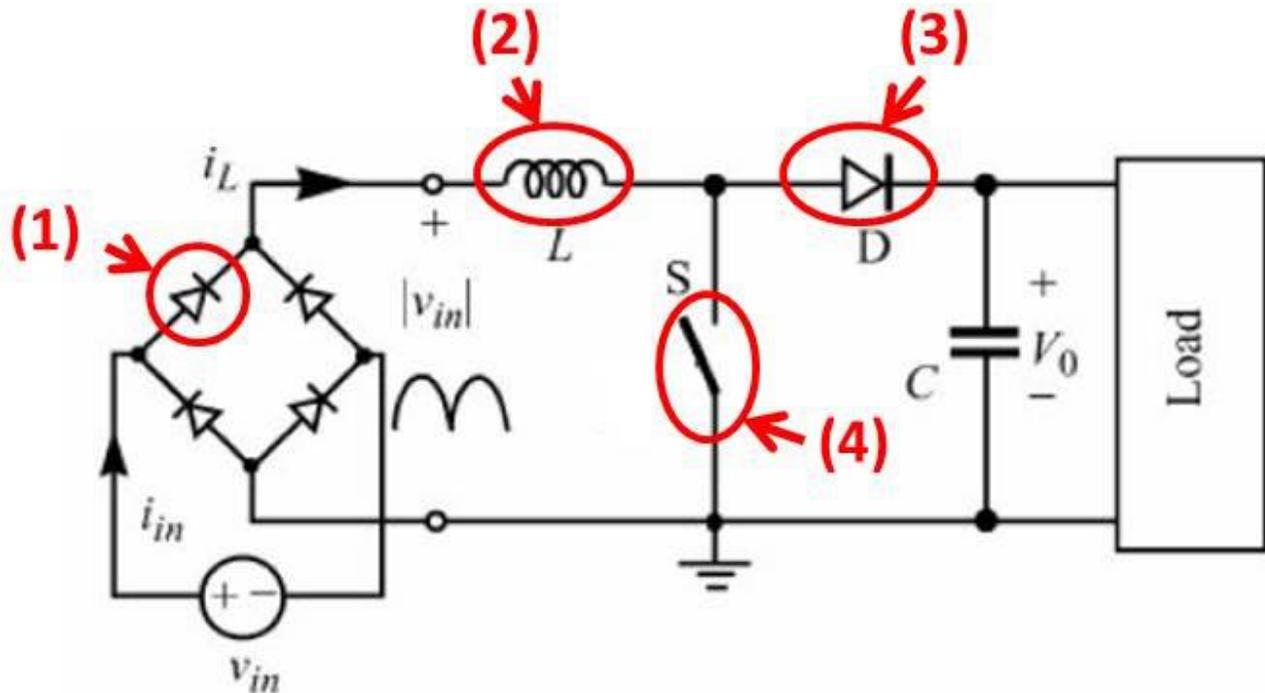
Figure 1. Typical Single-Phase Boost PFC Main Power Stage
