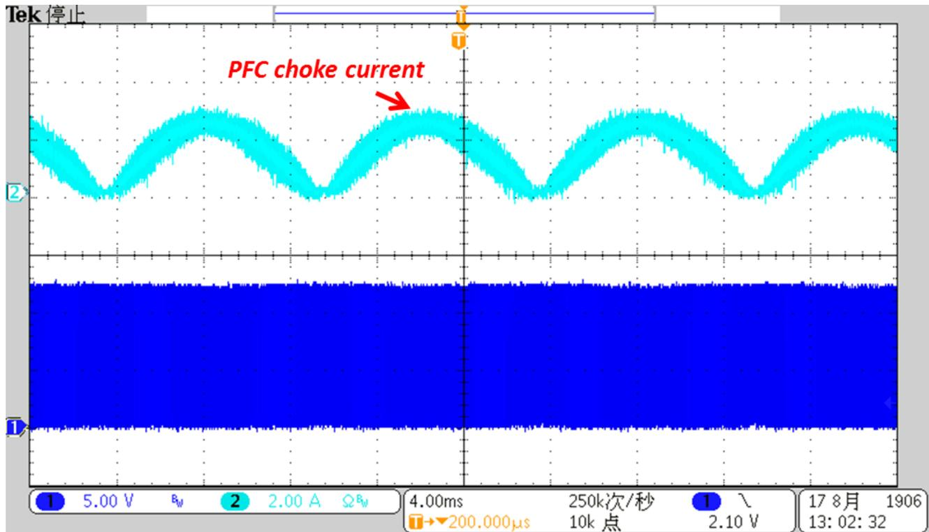
**Figure 2. Line-Frequency PFC Choke Current Under a 230-V<sub>AC</sub> Input**
