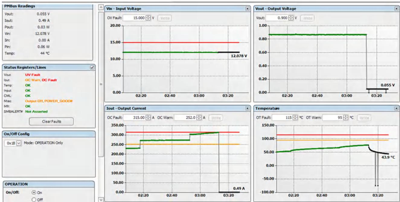
**Figure 3. Output Current Overcurrent Response – Warning at 252A, Latch off at 315A**
