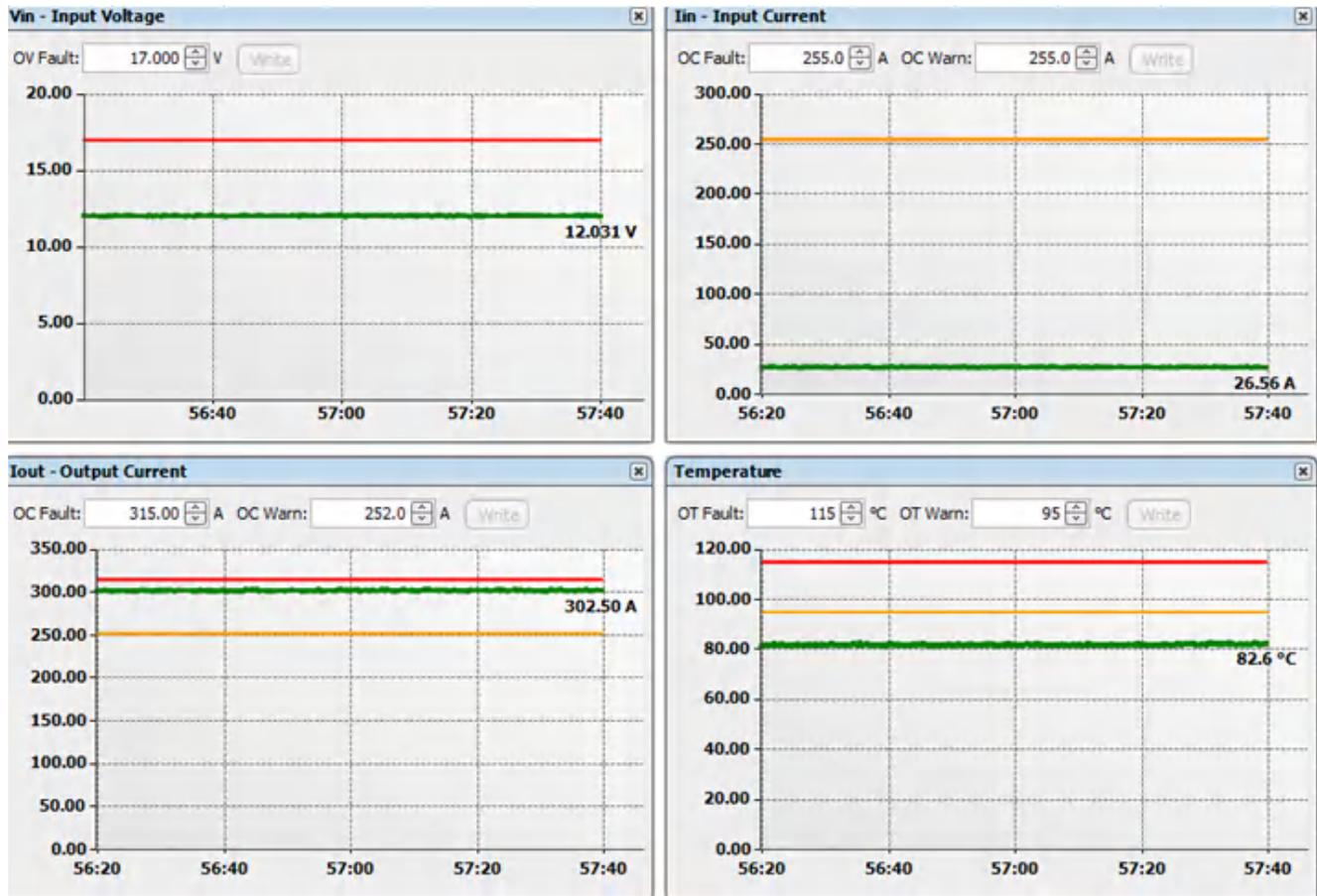
**Figure 5. PMBus Monitoring of the TPS53681'S Input Voltage, Input Current, Output Current and Temperature**
