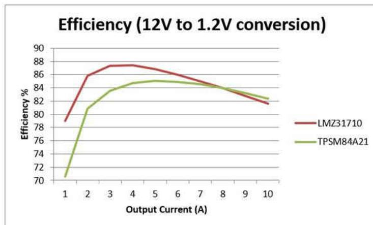
**Figure 2. Efficiency Comparison for a 12V-to-1.2V Conversion**
