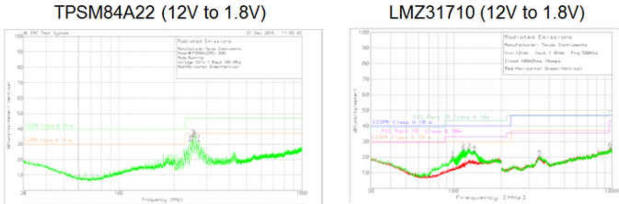
**Figure 5. Radiated EMI Comparison**
