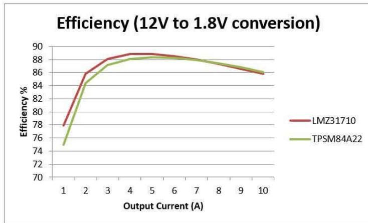
**Figure 3. Efficiency Comparison for a 12V-to-1.8V Conversion**
