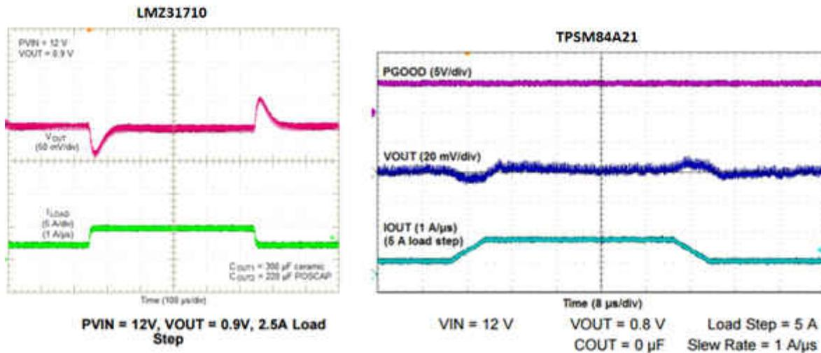
**Figure 4. Transient Response Comparison**
