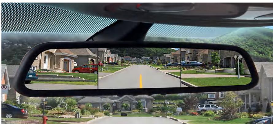
**Figure 1. Three-camera Mirror replacement/CMS Example**
