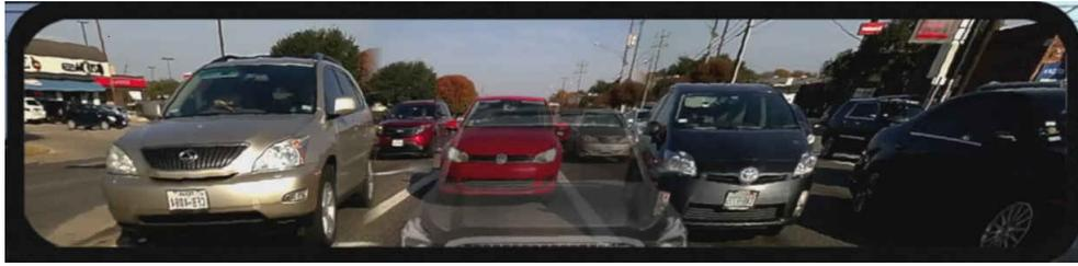
**Figure 2. Rear-stitched View Panorama (RSVP) Display, with Virtual Vehicle Graphic Overlay for Relative Positioning**
