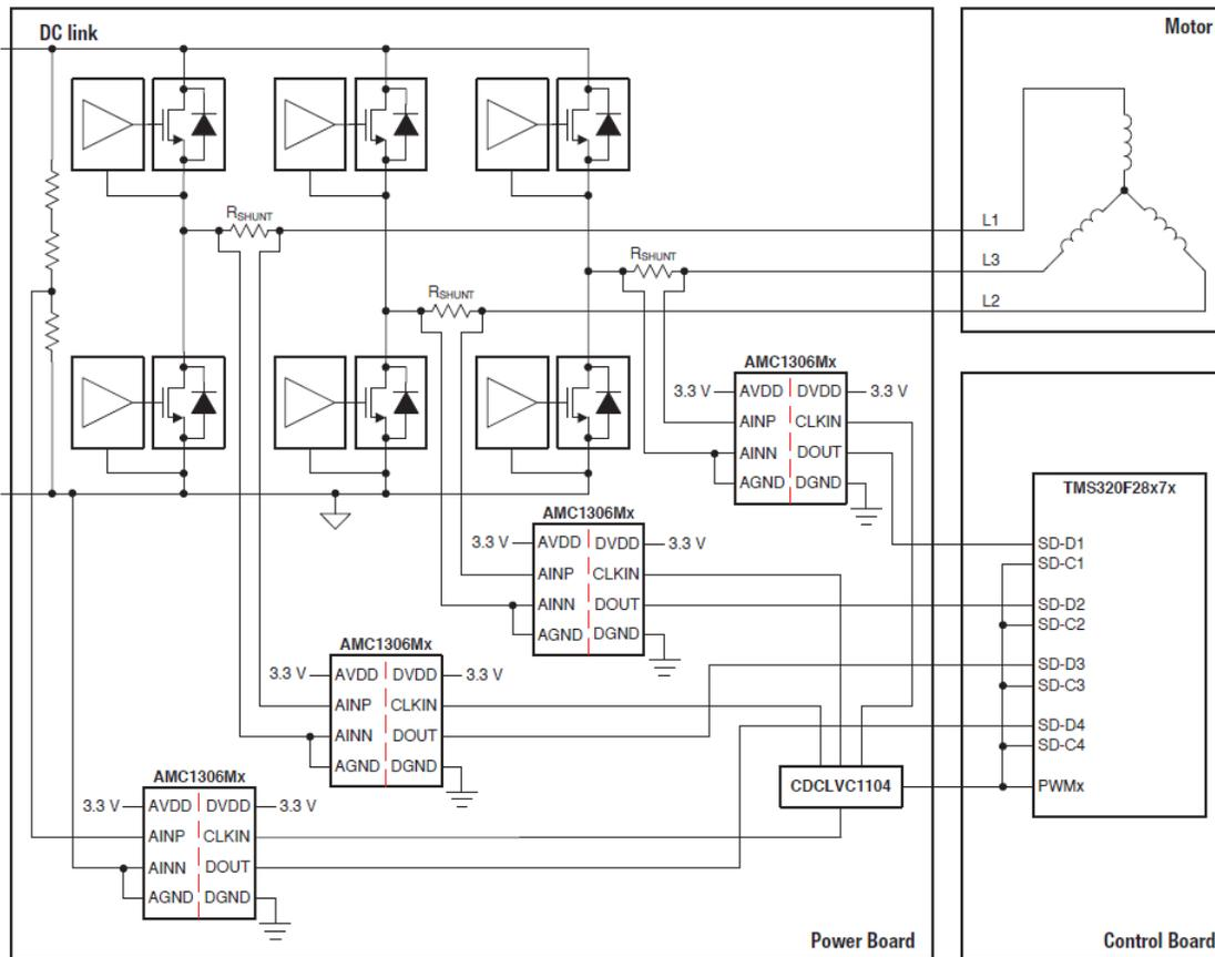
**Figure 1. Reinforced Isolated Phase Current-sense Reference Design with Small Delta-sigma Modulators**
