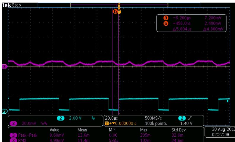
**Figure 11. Automotive 4V-36V Power over Coax Reference Design Final 2.8V Voltage Ripple**
