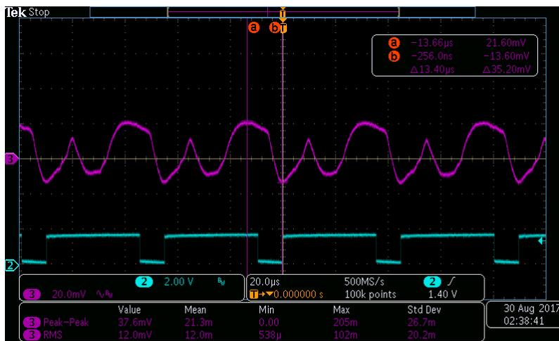
**Figure 5. 2.8V Voltage Ripple with Ferrite Bead – 35.2mV<sub>P,P</sub>**
