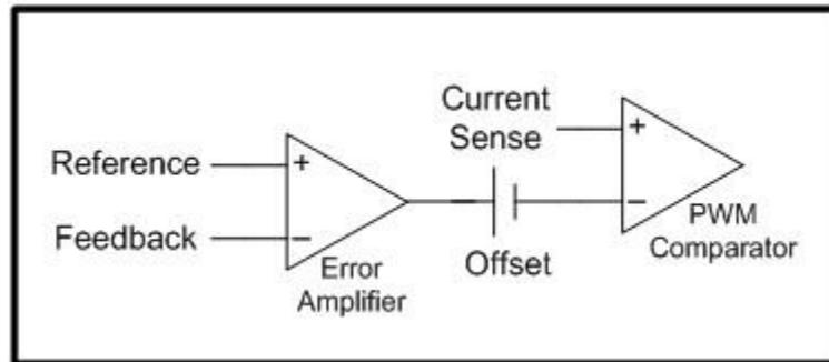
**Figure 1. Controller Block of a Boost Device**
