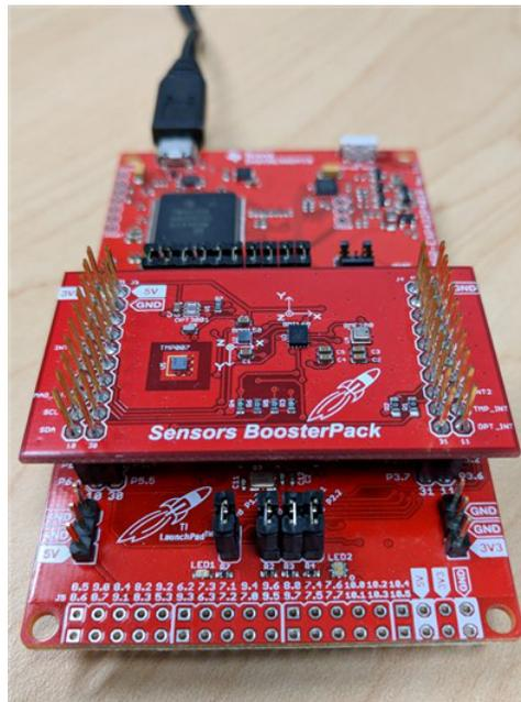
**Figure 2. MSP-EXP432P401R LaunchPad Development Kit and BOOSTXL-SENSORS BoosterPack Module with SimpleLink SDK Plug-in Support**
