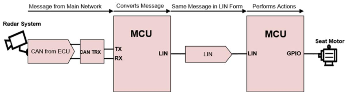
Figure 2. Diagram Showing a Message from a Car’s Radar Network Reaching a Remote Seat Motor via LIN
