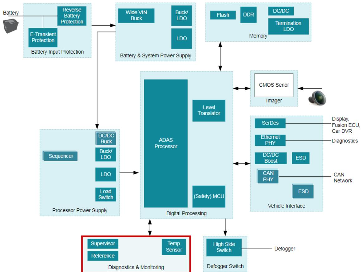
Figure 1. System Block Diagram for a Mono Front Camera
