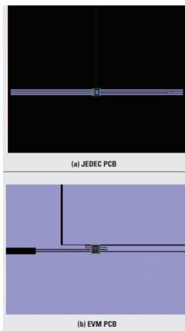
**Figure 2. The JEDEC PCB Uses Very Thin Amounts of Copper Connecting to the Device’s Pins**
