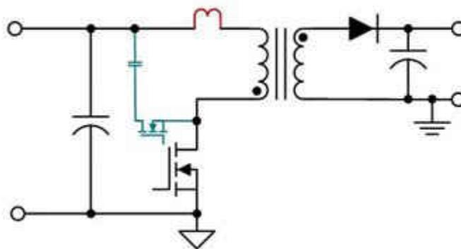
**Figure 1. Active Clamp Flyback with Leakage Inductance in Red and Active Clamp in Blue**
