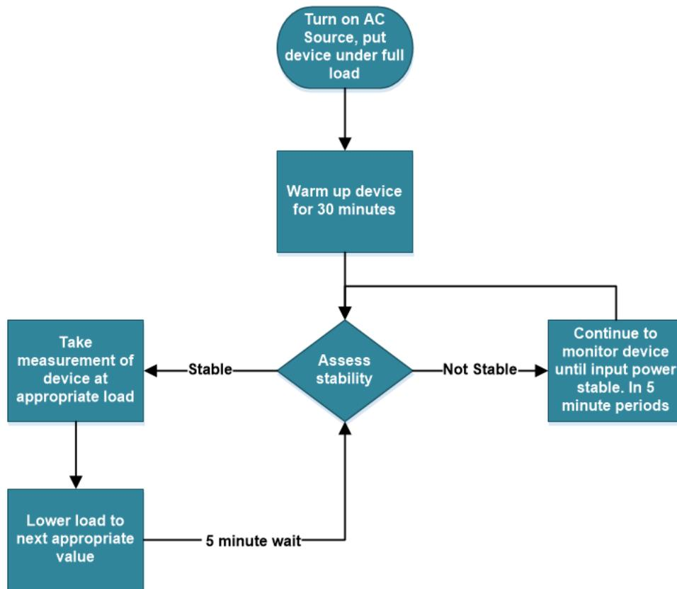
**Figure 3. Efficiency Measurement Procedure**
