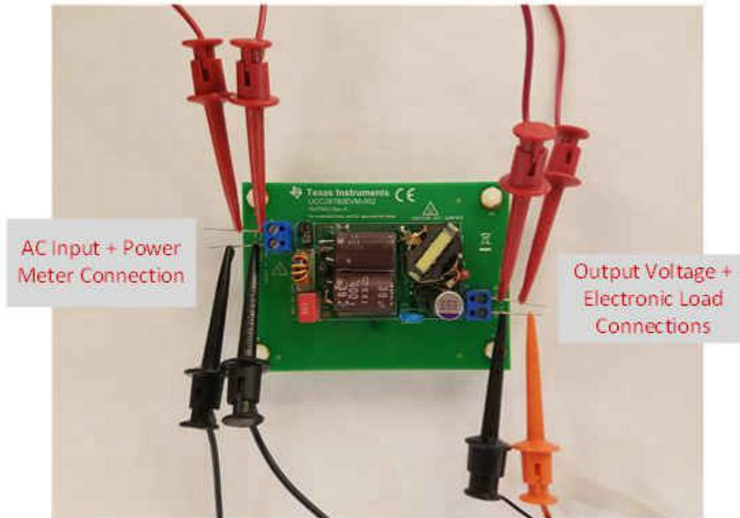
**Figure 2. Probe Connections for Efficiency Measurements**
