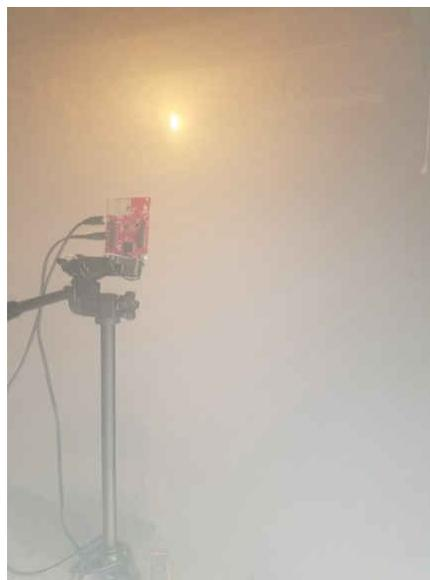
**Figure 4. mmWave Fine Motion Detection Can Function Even in Challenging Environments, Such as Rooms That Are Filled with Smoke and Sources of Heat.**
