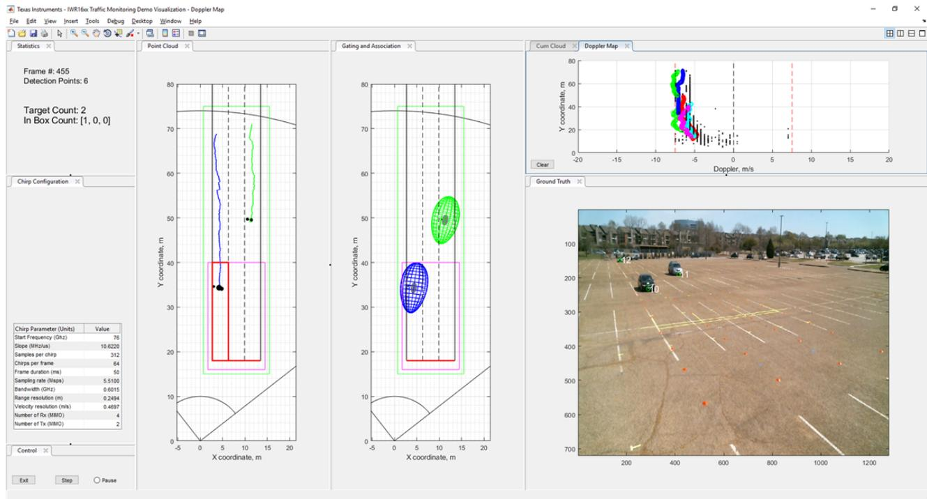
**Figure 2. The Graph on the Left Clearly Shows the Detection and Tracking of the Two Cars in the Picture Using the IWR1642**
