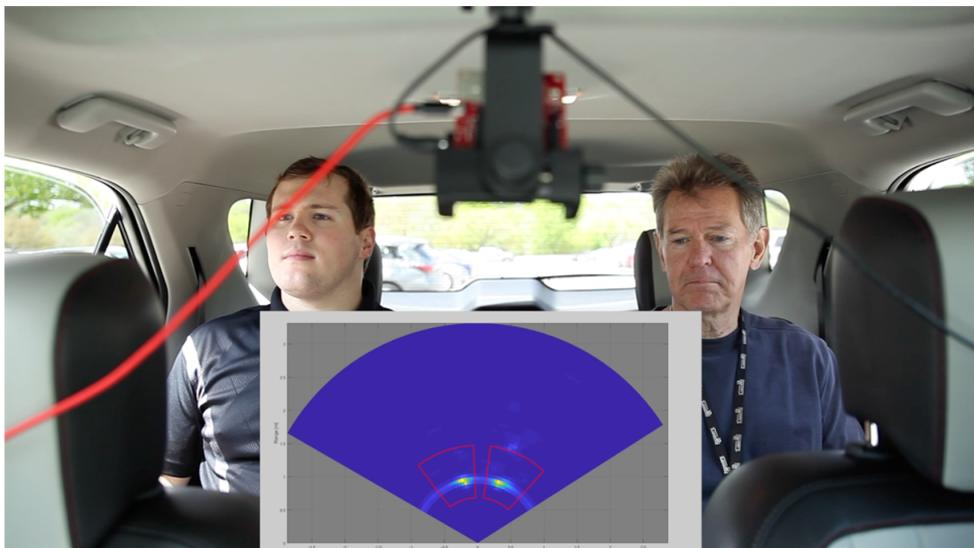
**Figure 2. TI’s mmWave Sensor Detects Two People Sitting in a Rear Seat**
