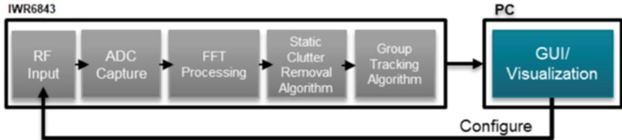
**Figure 2. The People Counting Demo Using the [IWR6843](#) Incorporates All Processing and Calculation Necessary for People Tracking and Static Clutter Removal Onboard the [IWR6843](#), Reducing System Complexity and Eliminating the Need for an External Processor**
