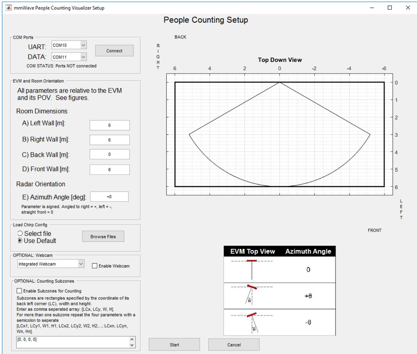
**Figure 3. You Can Use the PC Visualization Tool for the People Counting Demo to Configure the Area and Counting Zones for Detection; the MATLAB-based Source Code for This Tool Is Provided as Reference in TI Resource Explorer**
