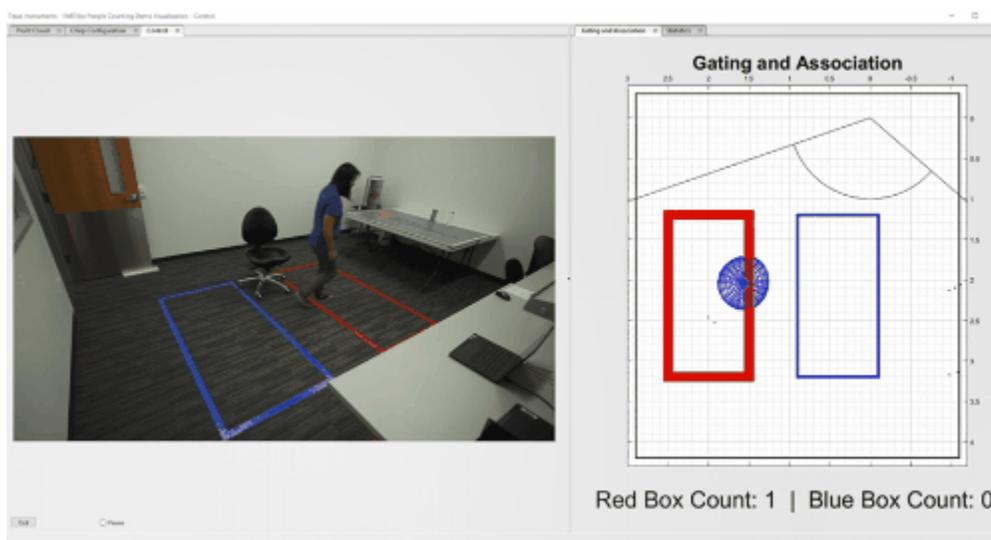
**Figure 1. An Example Indoor Location Output Generated from the mmWave Sensor, Which Is Tracking the Location of Multiple People Simultaneously Relative to the Two Boxes Indicated on the Ground**
