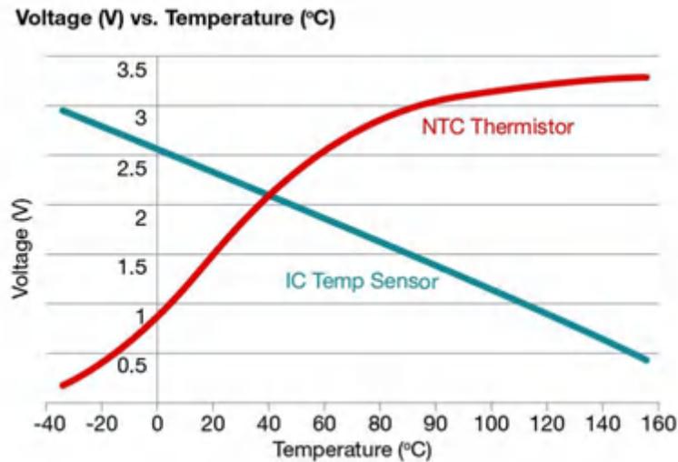
**Figure 2. NTC-based vs. Temperature Sensor Integrated Circuit (IC) Voltage Response**
