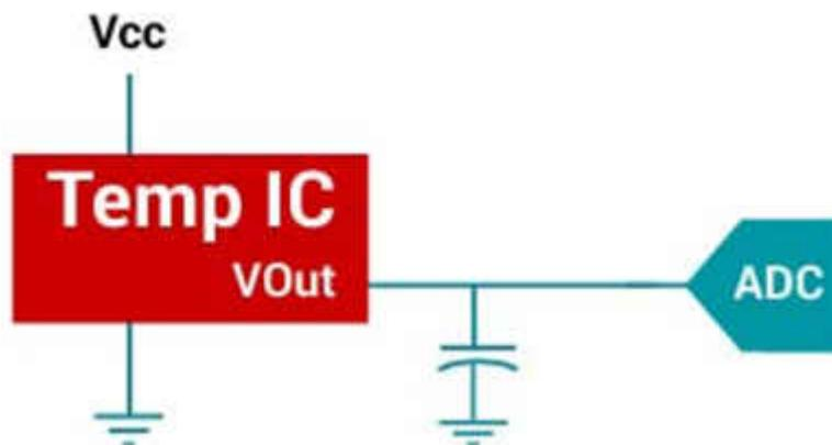
**Figure 3. Temperature-sensing IC circuit**
