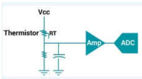
**Figure 1. Thermistor-based Temperature Monitoring**
