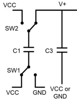
**Figure 3. The Diagram of Generating v+ Voltage (Cycle Two)**
