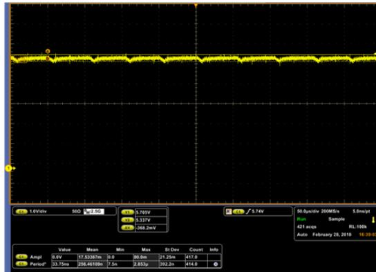
Figure 8. V+ Waveform, C1 = 0.01µF, C3 = 0.1µF
