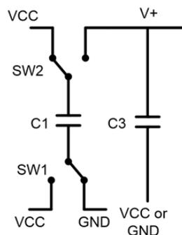
Figure 2. The Diagram of Generating v+ Voltage (Cycle One)
