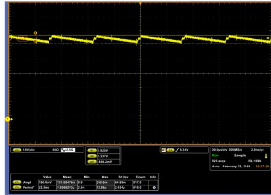
Figure 7. V+ Waveform, C1 = 0.1µF, C3 = 0.1µF
