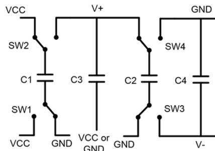
Figure 1. Charge-pump Circuitry Diagram
