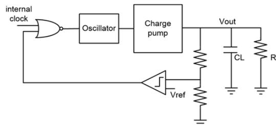
**Figure 4. The Regulator Circuitry Diagram**
