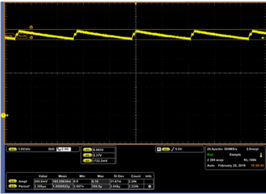
Figure 6. V+ Waveform, C1 = 0.47µF, C3 = 0.1µF
