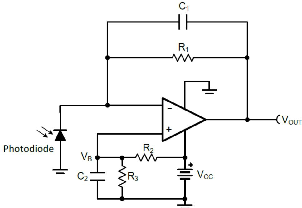
**Figure 1. Transimpedance amplifier configuration with a reverse-offset bias at the noninverting input**
