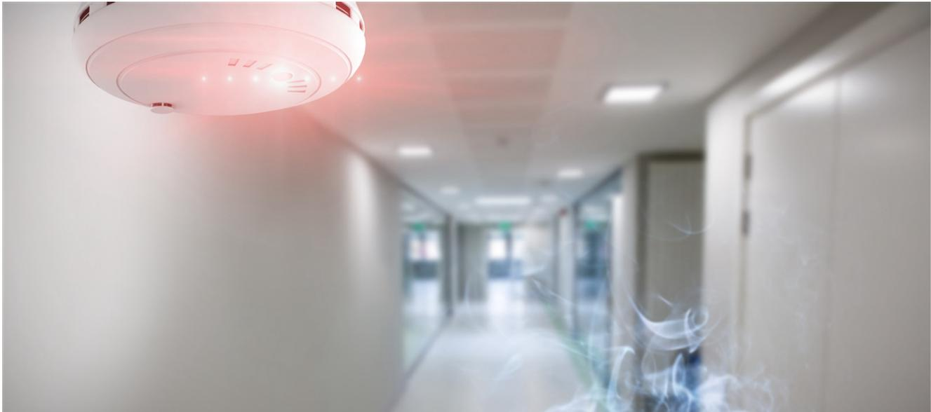
Thanks to modern-day electronics, designing these types of smoke detectors is simple, robust and cost-effective. When smoke detectors are AC-powered, they typically have 9V backup batteries. Thus, they have to be designed for the absolute lowest power consumption to reduce the size of the AC/DC power supply and increase battery life during backup.
