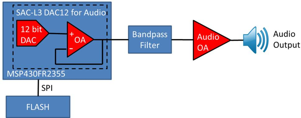
**Figure 3. Audio Application Using the MSP430 Smart Analog Combo**
