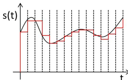
Figure 1. DAC Output Waveform
