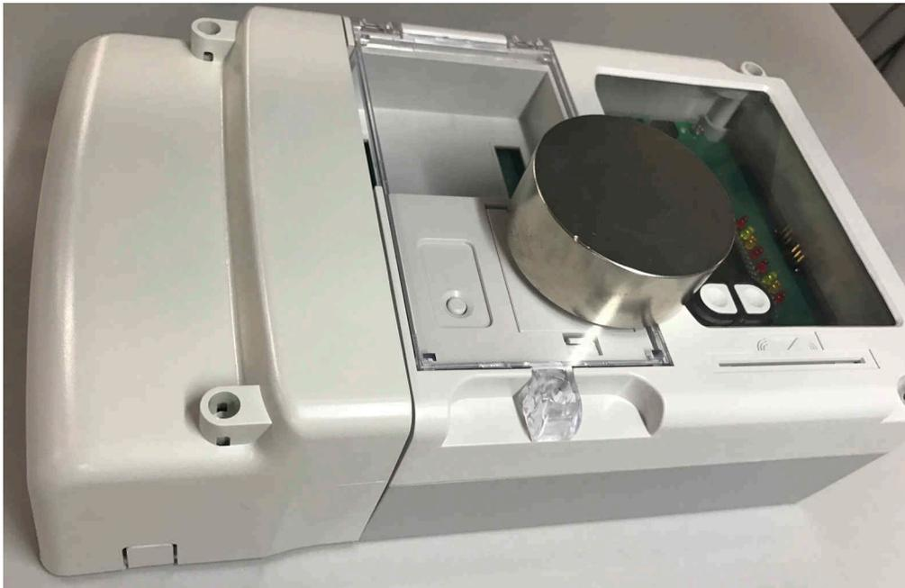
**Figure 1. A Tampering Magnet Applied to a Meter Case**
