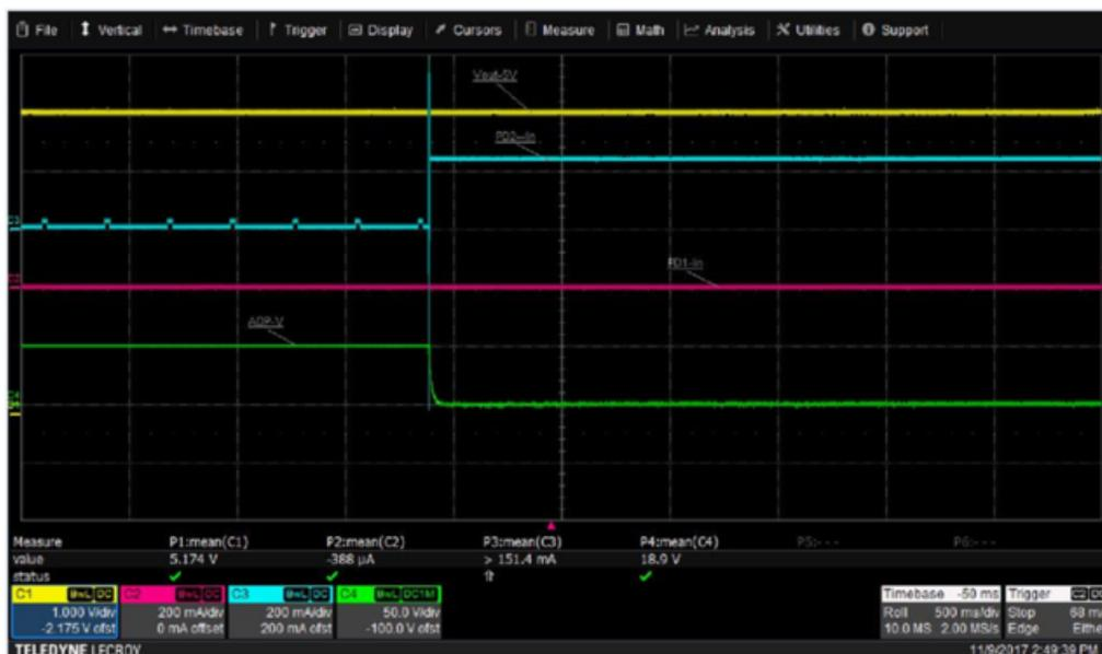
**Figure 2. Adapter and PoE Power Transition with Hitless Failover**
