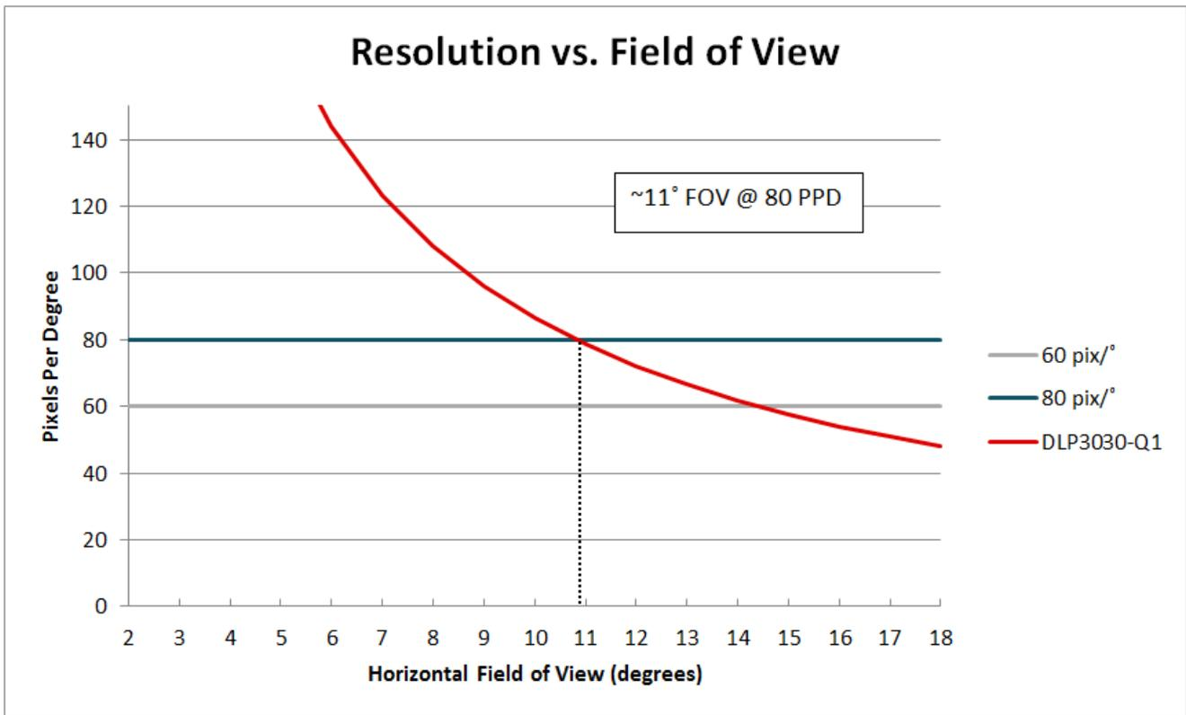
**Figure 4. Resolution vs. FoV for the DLP3030-Q1 Chipset**
