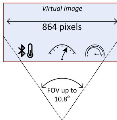
**Figure 3. Maximum FoV Supported by the TI DLP3030-Q1 Digital Micromirror Device (DMD) at 80 Ppd**
