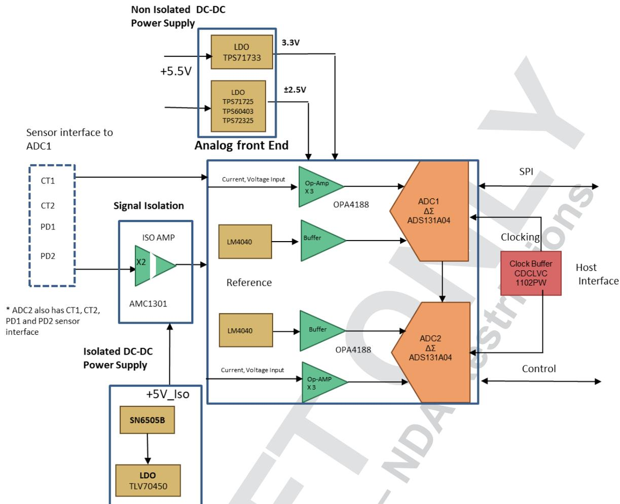
**Figure 2. Reference Design AFE Block Diagram**
