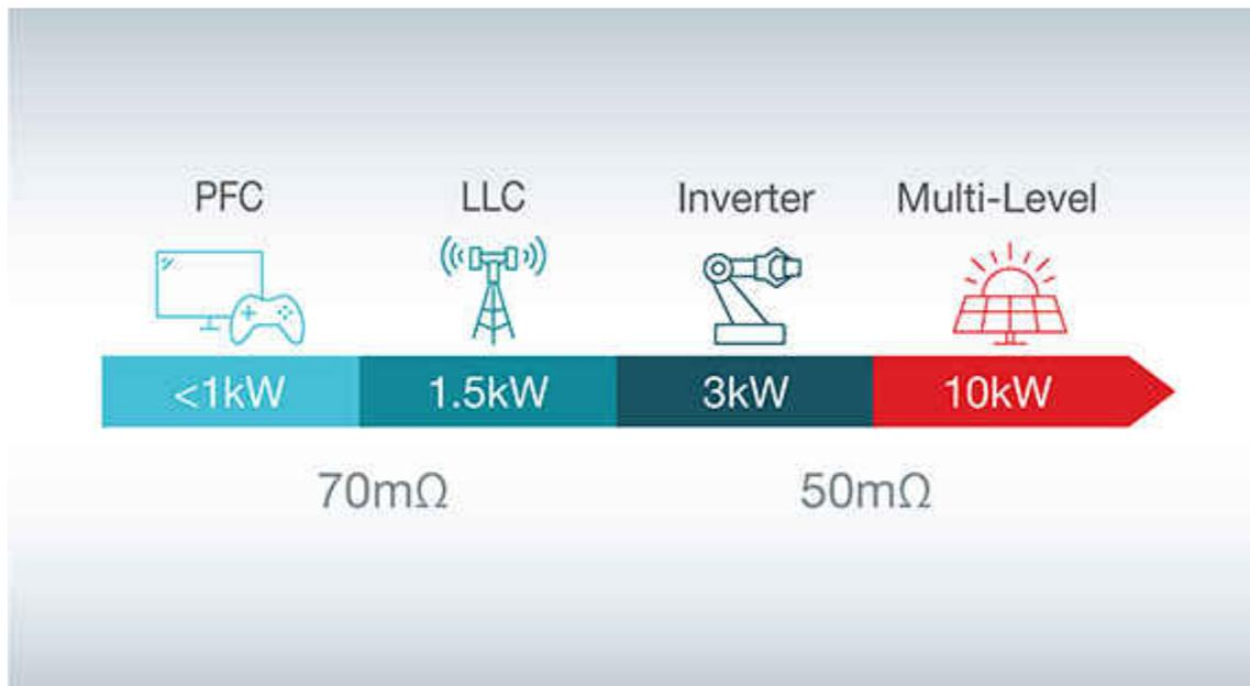
Figure 1. 70- And 50-mΩ GaN Devices in Typical Power Topologies
