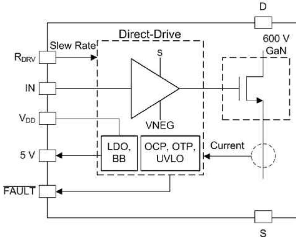
**Figure 2. Internal Device Structure for the LMG3410/LMG3411 Families, Including FET, Internal Gate Drive, Slew-rate Control and Protection Features**
