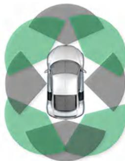
**Figure 1. mmWave Sensors Provide 360-Degree Sensing Capabilities around the Car to Enable Automated Parking Applications**
