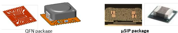
**Figure 5. Power module packages**
