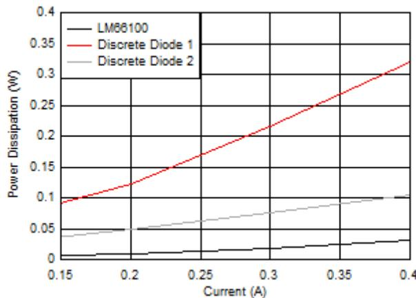
Figure 5. Power Dissipation LM66100 vs Discrete Implementation
