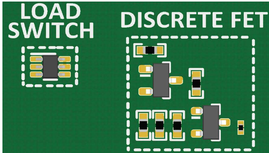
Figure 4. Load Switch vs Discrete FET-based Solution Size Comparison
