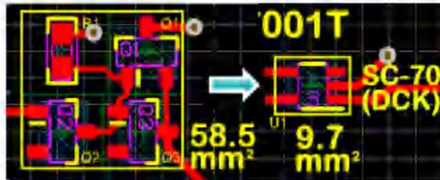
**Figure 3. Size Comparison between Discrete Push-pull Level Translation (Left) and the 2N7001T Implementation**
