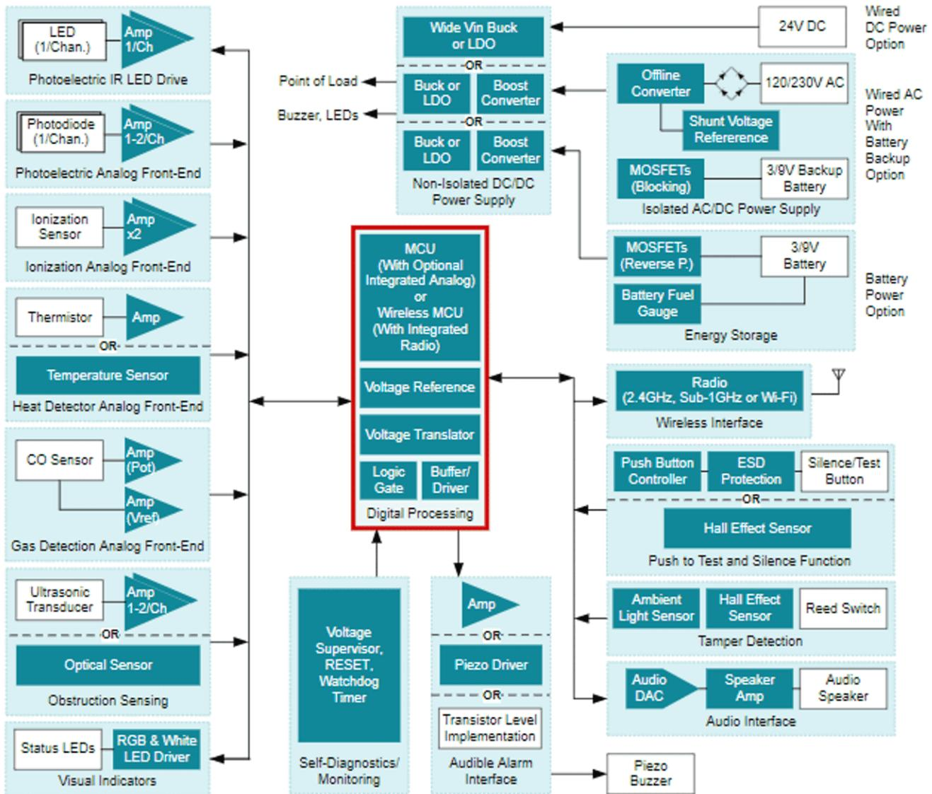
Figure 1. Residential Smoke and Heat Detector Design Block Diagram
