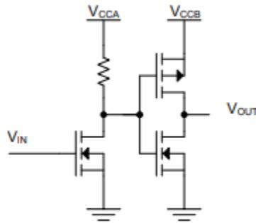
**Figure 2. Discrete Push-pull Level-translation Implementation**
