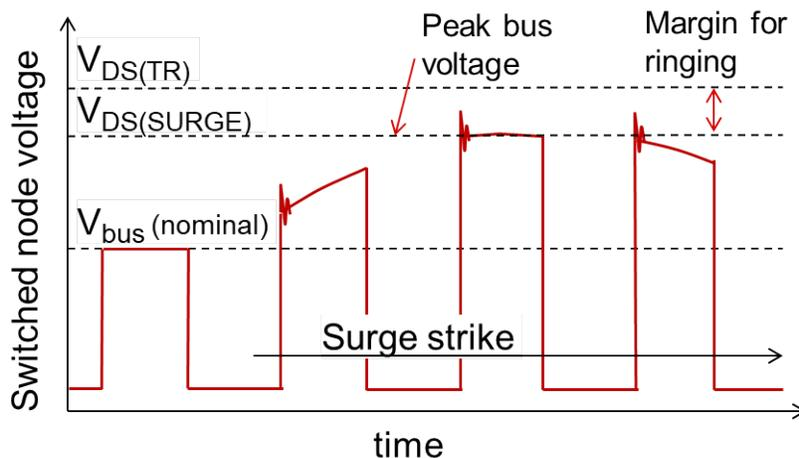
**Figure 1.** The surge rating parameter,  $V_{DS(SURGE)}$ , is the peak bus FET withstand voltage during operation when a surge strikes. Some GaN data sheets already have an off-state transient overvoltage parameter,  $V_{DS(TR)}$ , that serves to provide additional margin for ringing.
